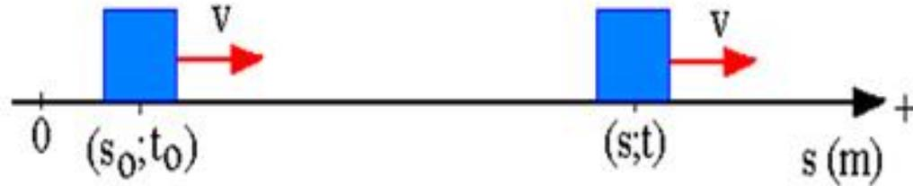
$$V_m = \frac{\Delta S}{\Delta t} \quad \rightarrow \quad V_m = \frac{S - S_0}{t - t_0} \quad \rightarrow \quad S = S_0 + v \cdot t$$
